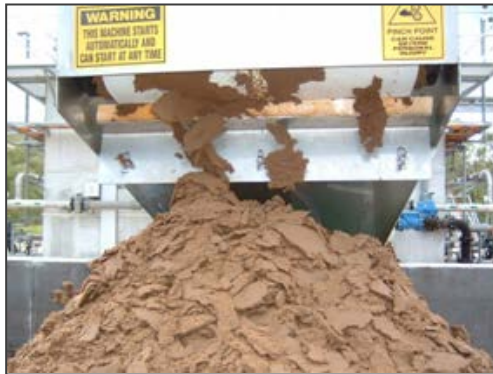
QUALITY LANDFILLABLE FILTER CAKE DISCHARGING FROM THE V-FOLD.
