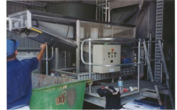
Direct discharge of overflow from Induced Air Flotation to a V-FOLD without additional polyelectrolyte
