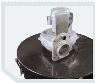
CLOSE-UP OF BLOWER WITH ADJUSTABLE DAMPER
